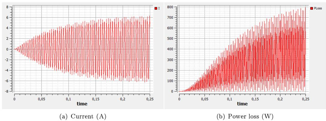
Figure 6: Current (a) and dissipated power (b) of the parametric circuit for frequency  $f = 0.97 f_0$ .
