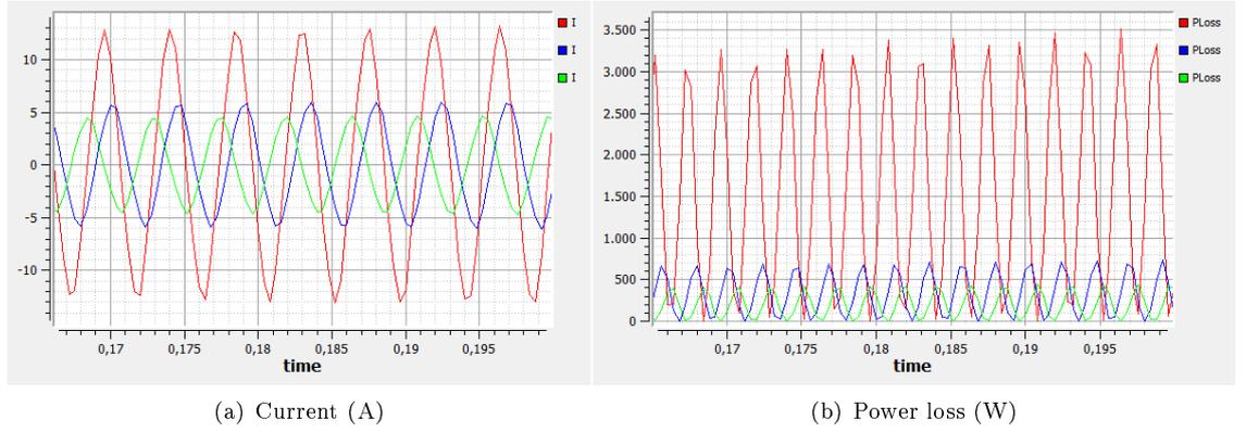
Figure 7: (a) Currents for different phase shifts between  $U$  and  $C_{eff}$  with  $f = 0.97 f_0$ . red:  $\varphi = -\pi/2$ , blue:  $\varphi = 0$ , green:  $\varphi = \pi/2$ .
