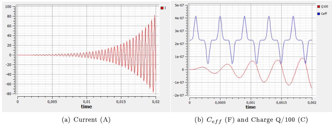
Figure 8: (a) Current for model with  $\sin^7$  pulses,  $f = 1.07 f_0$ ,  $\omega_1 = \omega_0$ .
