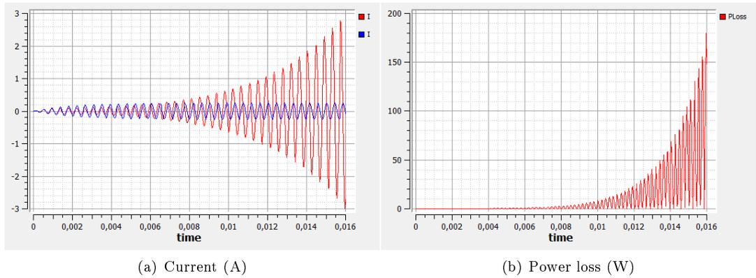
Figure 5: (a) Current of the parametric circuit described by parameters of Eqs.(28-36). For comparison: current amplitude of the original free oscillating circuit of Fig. 3a (blue curve).
