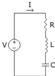
Figure 2: Serial resonance circuit with driving voltage [2].
